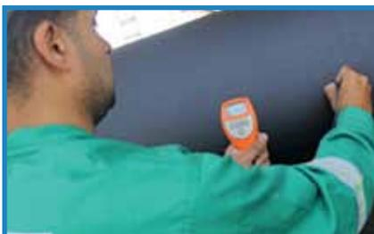
BITUMEN COATING THICKNESS
